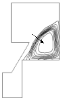
(e) \alpha = 30^\circ , z = 3 mm, v = 5 m/s Diameter of front face = 10 mm
